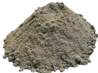
Hot Patching Mass
